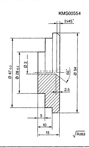
Improvised tool for pressing out needle bearing in armature
